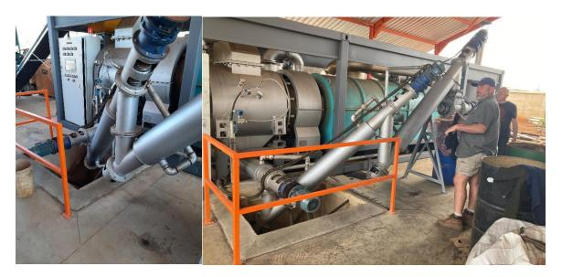
The installation to produce Biochar is now ready! This pilot unit is a machine that is able to process about 10 tons a day of organic reststreams. This results in more than 3 tons Biochar a day. Biochar can be used as soil improvement or as raw material for briquettes, building materials or other aspplications.
